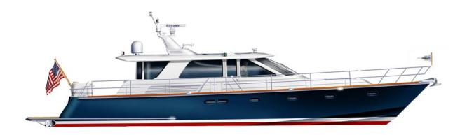
Length (Hull): 68'-5 1/2" (20.87 m) Length Overall with swim platform: (LOA) 72'-11 1/2" (22.24 m) Waterline Length (DWL): 60'-7 1/2" (18.48 m) Molded Beam: 19'-6" (5.95 m)Draft with Props: 5'-4 1/2" (1.65 m) Air Draft: 21' (6.42 m) Displacement (Half Load): 110,000 lbs. (49.9 Tons)
